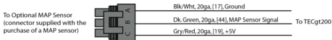
Figure 40: MAP sensor wiring.
