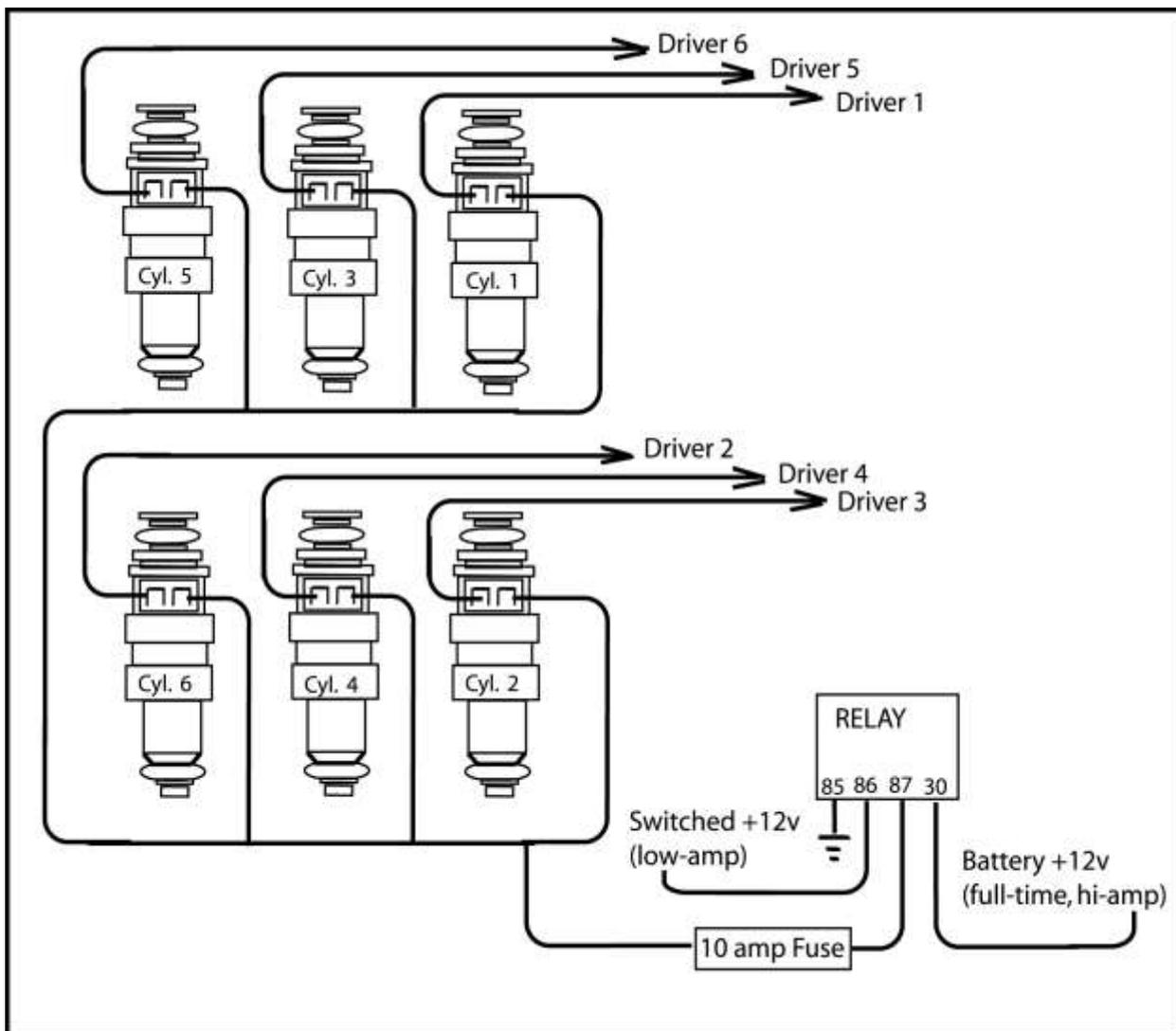
**Figure D.2.3 :** 6-cylinder full-sequential injection wiring for a 1-6-2-4-3-5 firing order.
