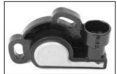
The throttle position sensor should have a resistance of roughly 10kΩ measured across the +5V and Ground terminals. To determine the pin out of an unknown TPS, follow the instructions below (you will need an ohmmeter):
