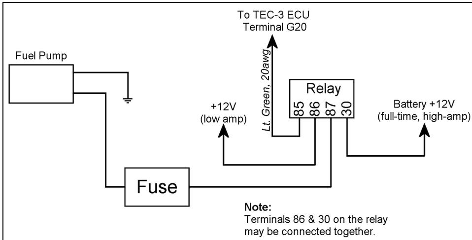
**Figure F.3. 1 :** Fuel pump relay wiring.
