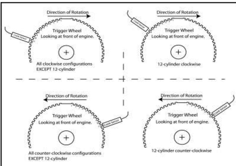
**NOTE:** 12 Cylinder applications require that the center of the sensor be aligned with the trailing edge of the 8<sup>th</sup> tooth.
