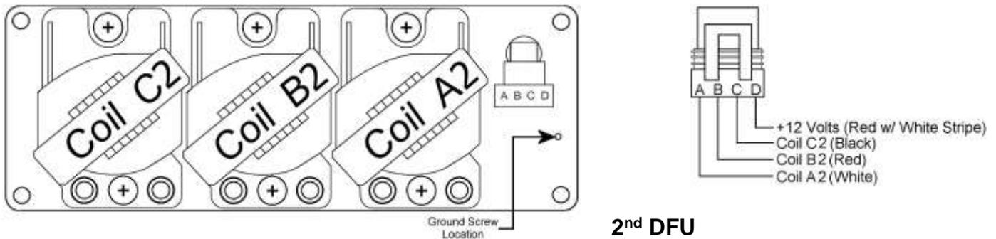
**Figure C.2. 5 :** 12-Cyl and Dual Plug 6-cyl DFU setup. When used on these applications, the first DFU will have coils A1, B1, and C1, and the second DFU will have coils A2, B2, and C2.
