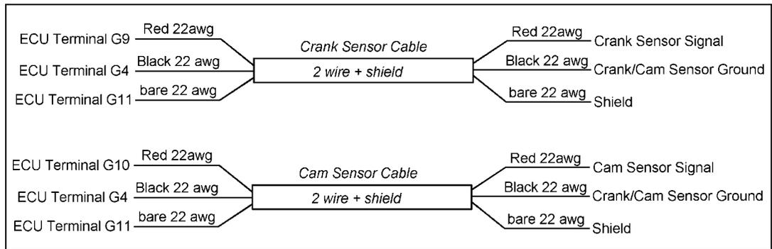
**Figure A.4.4:** Wiring layout for crank and cam sensors. Note that the Cam Sensor is only used on full sequential applications. It is NOT used on applications using the 120(-4) tooth cam trigger wheel with no crank trigger.
