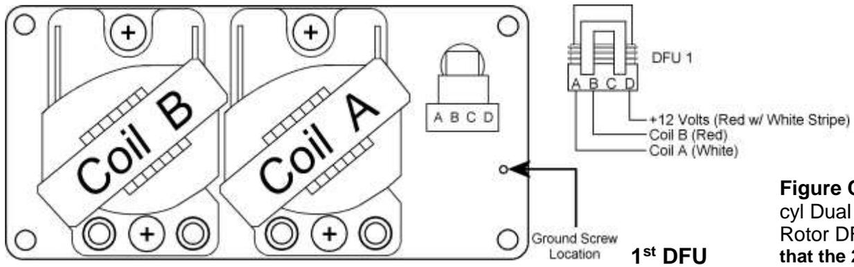
**Figure C.2.3 :** 8-Cyl, 4-cyl Dual Plug, and 2-Rotor DFU Setup. **Note that the 2<sup>nd</sup> DFU coils will not be labeled C and D from Electromotive.** When the 2<sup>nd</sup> DFU is wired as shown, the coil labeled "A" will fire coil output "A2." The coil labeled "B" will fire coil output "B2."
