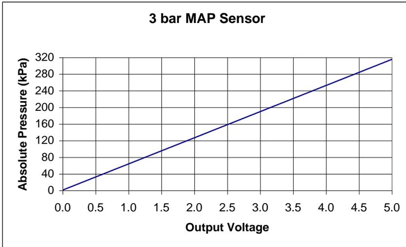
**Figure G.1. 4 :** 3-Bar MAP sensor output voltage.
