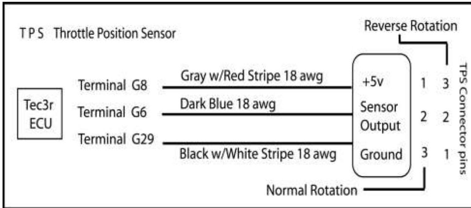
**Fig G.2.7 :** Proper throttle position sensor wiring
