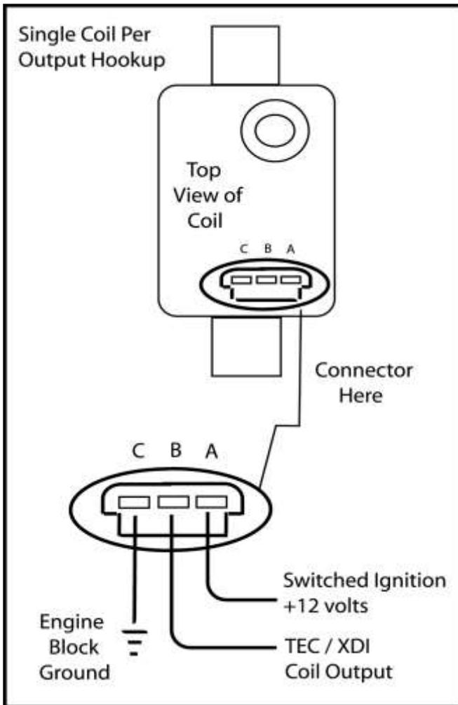
**Figure C.3.1** : 2-Rotor (Mazda 12A and 13B) coil setup. 4 of these coils will be required for leading and trailing plugs.
