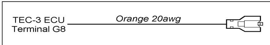
**Fig G.6.1** : Knock sensor wiring.
