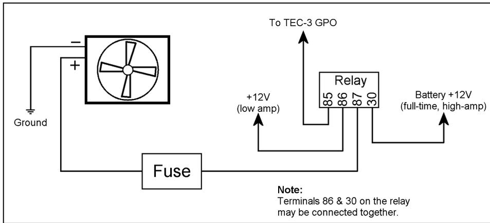
**Fig. F.4. 1 :** Electric radiator fan wiring.
