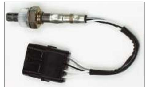
When installing the sensor, take care not to run the wires on the exhaust. This will obviously melt the wires once exhaust temperatures rise.
