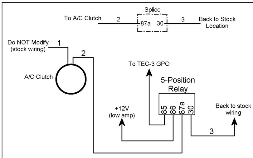
**Fig F.4. 3 :** Air conditioner control wiring. Note that the relay simply splices into either of the two wires on the A/C clutch with terminals 30 and 87a. When activated, the A/C control will break the (normally-closed) connection between 30 and 87a by grounding pin 85.
