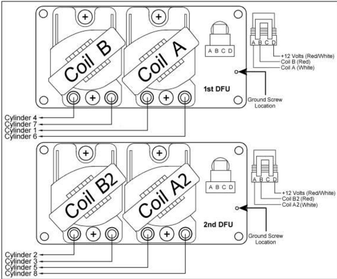
**Figure C.4.3 :** Typical GM 8-cylinder DFU wiring. Firing Order 1-8-4-3-6-5-7-2 depicted here. Remember, 8-cylinder setups fire the coil channels in the order of A<sup>1</sup>-A<sup>2</sup>-B<sup>1</sup>-B<sup>2</sup>.
