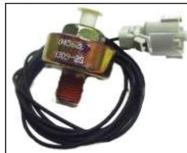
drive, but the datalog indicates that there was knock in the upper rpm/light load area, mechanical noise may be false triggering the knock sensor.
