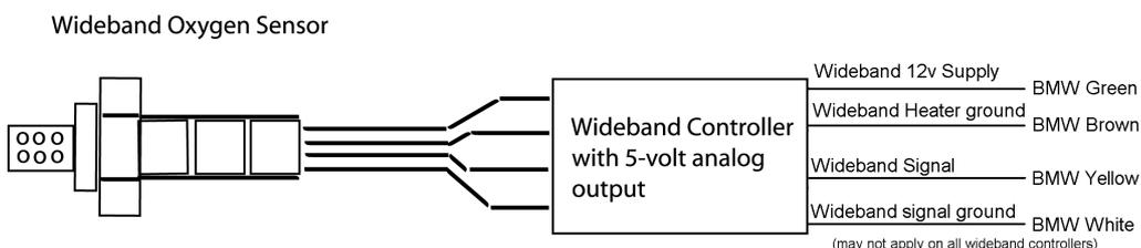
The factory pre-cat narrow band O2 connector can be repurposed for wiring in a wideband O2 sensor. The wideband module can pull 12v and power ground from the EGO heater leads (Green and Brown) and has a signal ground available on the White wire if needed. Finally the 0-5v output of the wideband module connects to the Yellow wire (See the chart below). The TECm would then need to be configured to use a Wideband O2 sensor in your engine calibration.
