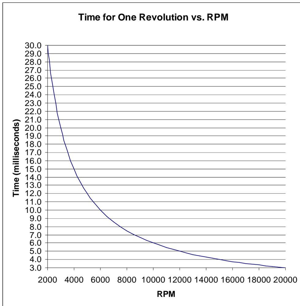
Figure: Time between revolutions for various engine speeds.
