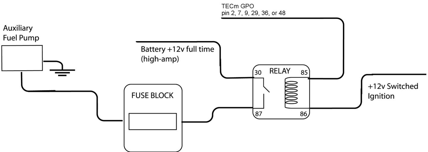
Figure H.2.4: Auxiliary fuel pump wiring
