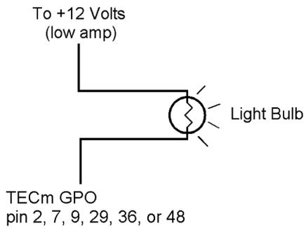
Figure: Shift light wiring.
