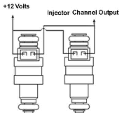
Figure: Parallel wiring of fuel injectors.
